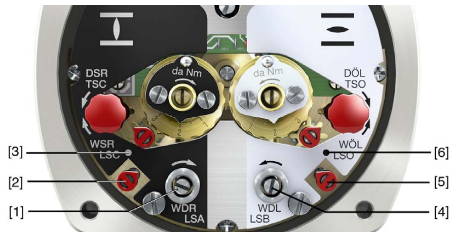
Figure 35: Setting elements for limit switching
