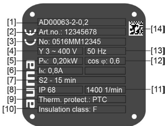
Figure 3: Motor name plate (example)
