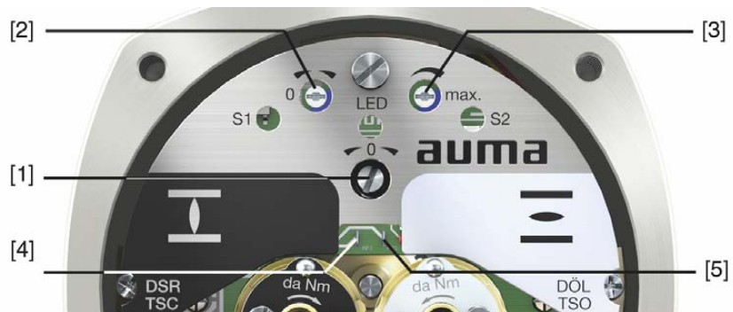
Figure 33: View on control unit when switch compartment is open
