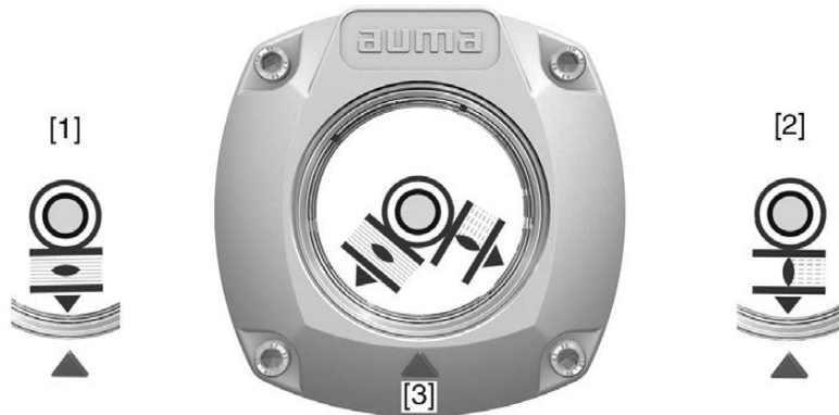
Figure 26: Mechanical position indication via indicator mark on cover
