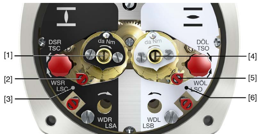
Figure 28: Setting elements for limit switching
