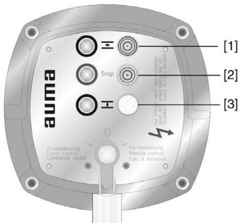
Figure 30: Local controls with indication lights
