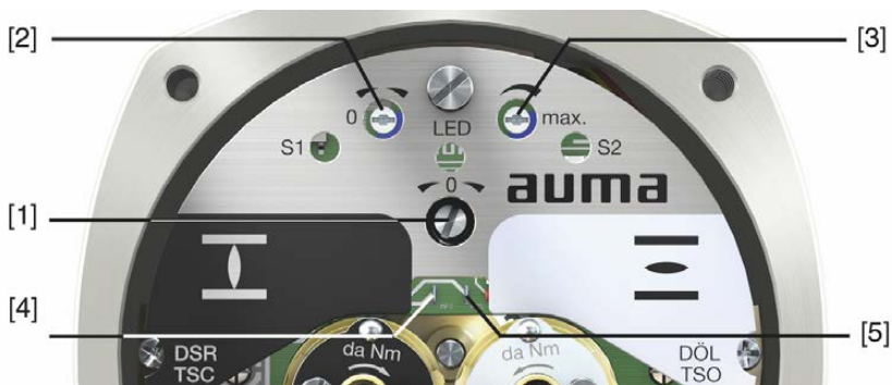
Figure 40: View on control unit when switch compartment is open
