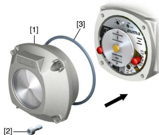
Figure 42: Close switch compartment
