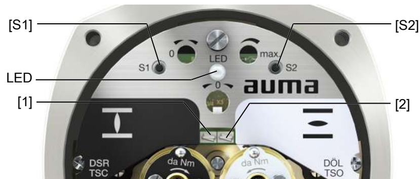
Figure 45: View on control unit when switch compartment is open
